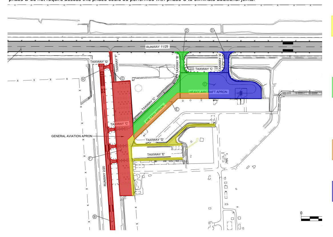
Phase A - General Aviation Apron; complete top lift paving prior to starting work on phase B. Provide temp striping and tie downs prior to starting on phase B. During construction provide two temporary tie downs near the intersection of taxiway C and B as directed by the airport manager. Maintain a 50 FT wide temporary access taxiway along the lease lots and taxiways D and E that will be paved in phase B.
